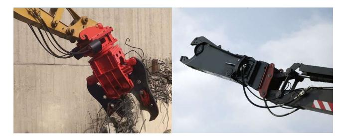
**Combi-Crusher:** Demolition of mixed concrete/iron structures or in strongly reinforced concrete.
